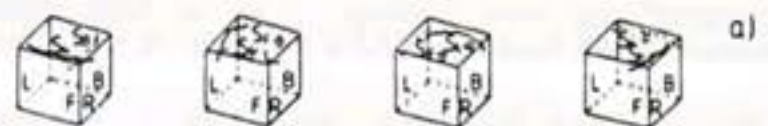
(a) The four basic phases of operation of the oscillatory chamber. R, L, F, B — the plates of the chamber that together form two cooperating oscillatory circuits; SR-L, SF-B, SL-R, SB-F — the electric sparks that appear in succession during one full cycle of oscillation.
